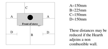
The stove surfaces must have a minimum distance away from any combustible materials as listed in the technical data section of this manual.
