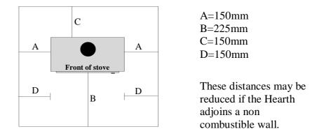
The stove surfaces must have a minimum distance away from any combustible materials as listed in the technical data section of this manual.
