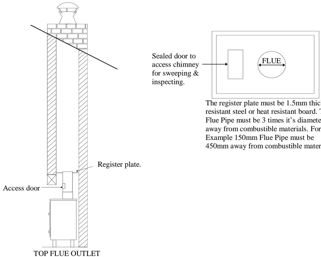
If the chimney is not sound, i.e. found to be leaking after a smoke test then the chimney must either be repaired or a flexible liner may be used, ensure the liner is the correct type for Multi-Fuel applications. See diagram below:
