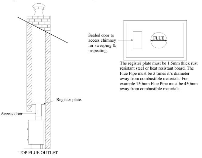
If the chimney is not sound, i.e. found to be leaking after a smoke test then the chimney must either be repaired or a flexible liner may be used, ensure the liner is the correct type for Multi-Fuel applications. See diagram below:
